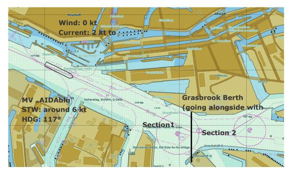
Figure 10: Exercise area and environmental conditions in Port of Hamburg for berthing scenario, divided into two sections for planning the manoeuvres
