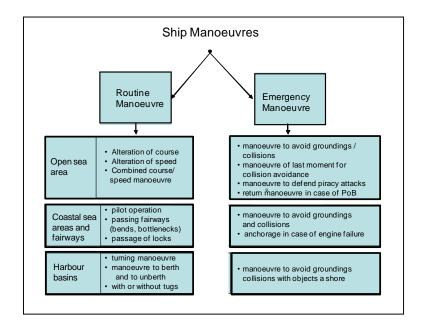
Figure 9: Systematization of ship manoeuvring
