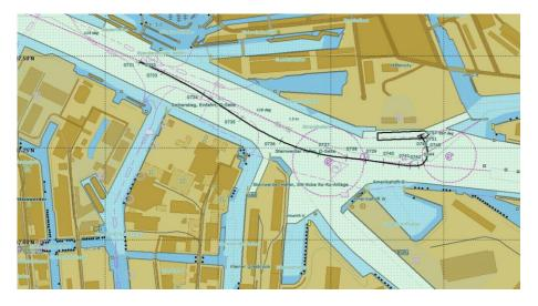
**Figure 14:** Result of manoeuvring training in ship handling simulator for a trainee with conventional preparation and no support by fast time simulation (Total Manoeuvring Time about 20 min)
