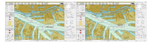
**Figure 12:** Final part of the manoeuvring plan: Left MP4 - The vessel is stopped and the heading is chosen in that way, that all handles can be set in zero position. Right: MP5 / MP6: the ship is already brought to the berth
