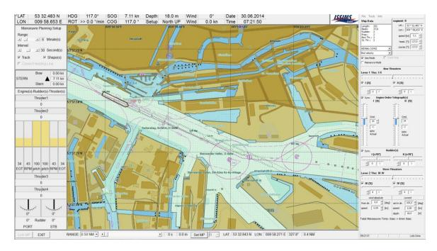
**Figure 11:** MPO: Initial position: The prediction already shows that the ship would drift slightly to portside due to the set handle positions.
