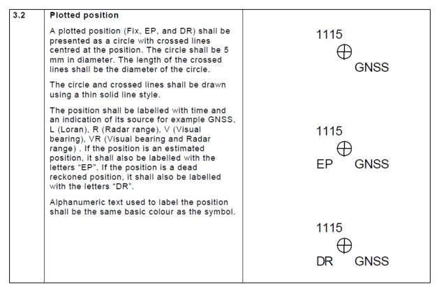
Figure 3.10 – Portrayal of ship's position. Information on time of fix and source of fix may be displayed.
