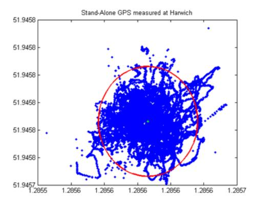
Figure 3.4 – GPS positioning error.
