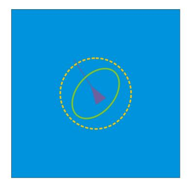
Figure 3.5 – Horizontal Protection Level (green ellipse) and Horizontal Alert Limit (yellow dashed circle), represented by ellipses around the vessel indicator (purple). This configuration indicates positioning is good and can be relied upon; HPL<HAL.
