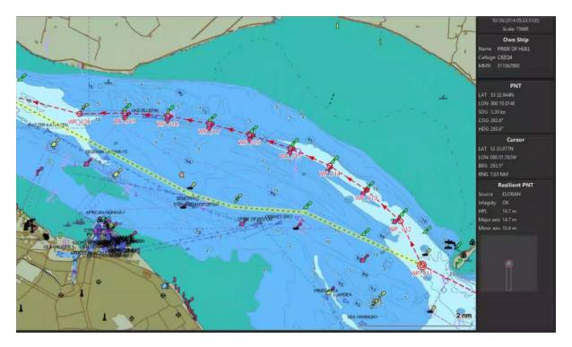
Figure 3.8 – EPD showing Resilient PNT display panel in the lower right.
