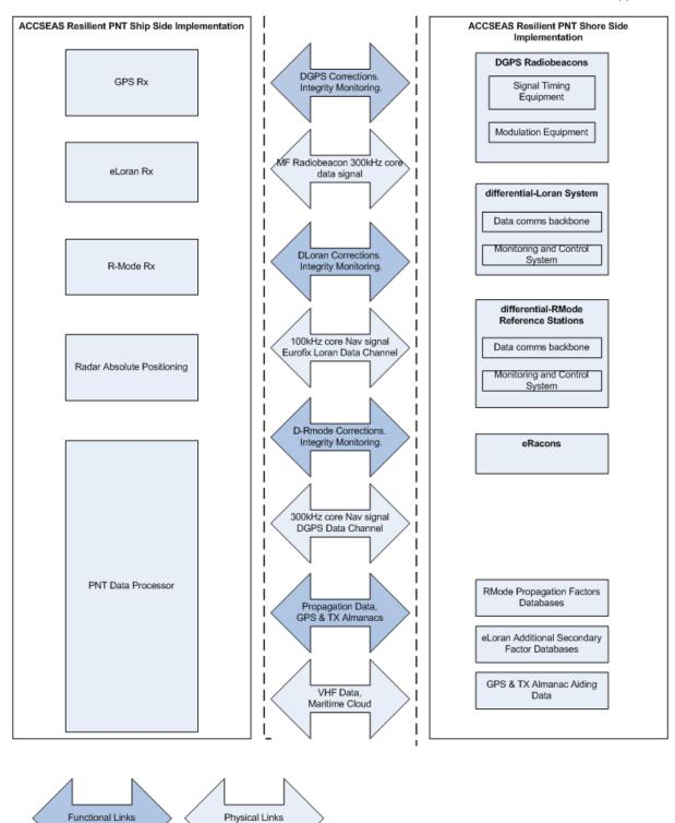
Figure 3.2 – Organisation of ship-side and shore-side components of the Resilient PNT system with Functional and Physical Data Links.
