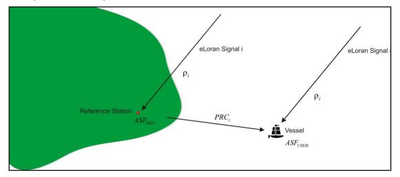
Figure A.5 – Principle of operation of differential-Loran.
