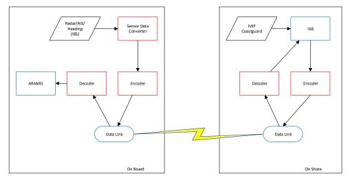
Figure 6- Test system software components.
