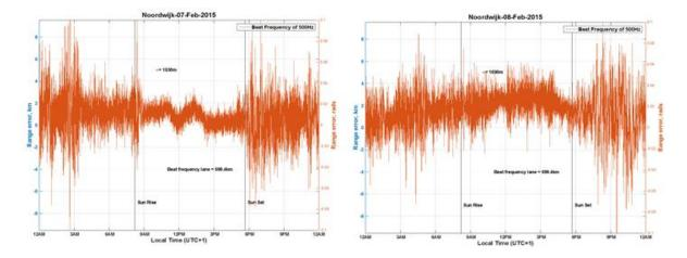
Figure E.4 - R-Mode Range Error of beat frequency as hourly average over time.
