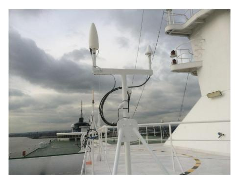
Figure 12 - GPS (right) and combined eLoran/DGPS radiobeacon antenna (left) installed on the Pride of Hull.
