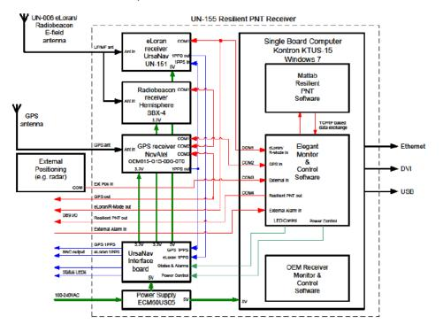
Figure 2 - Block diagram of the ACCSEAS Multi-Source Receiver.
