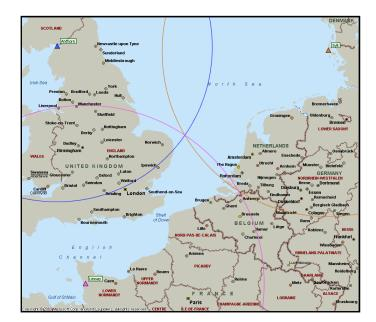
Figure A.1 - Example of circular positioning using Anthorn, Lessay and Sylt.
