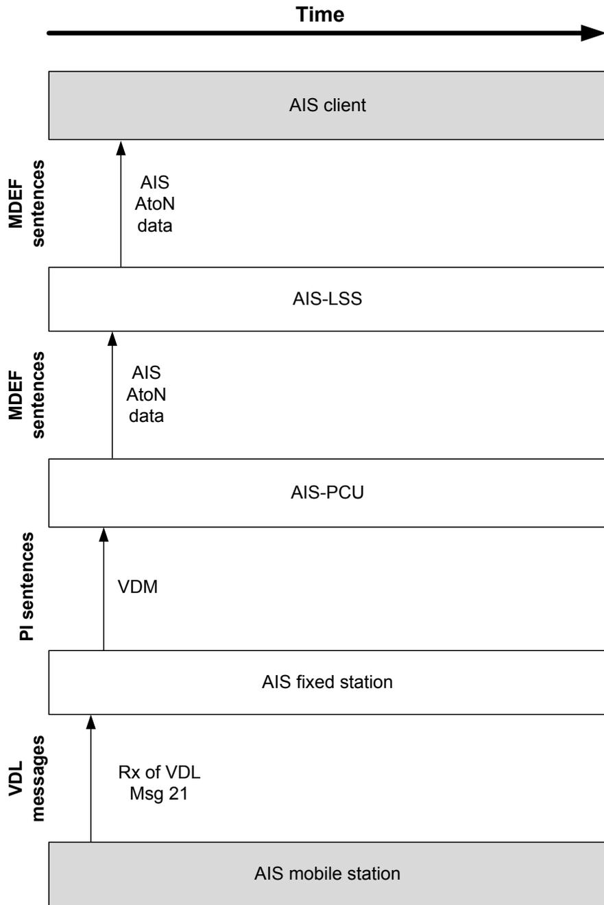
Figure 9 Interaction & data flow model for external BAS ATON\_DAT in Rx mode
