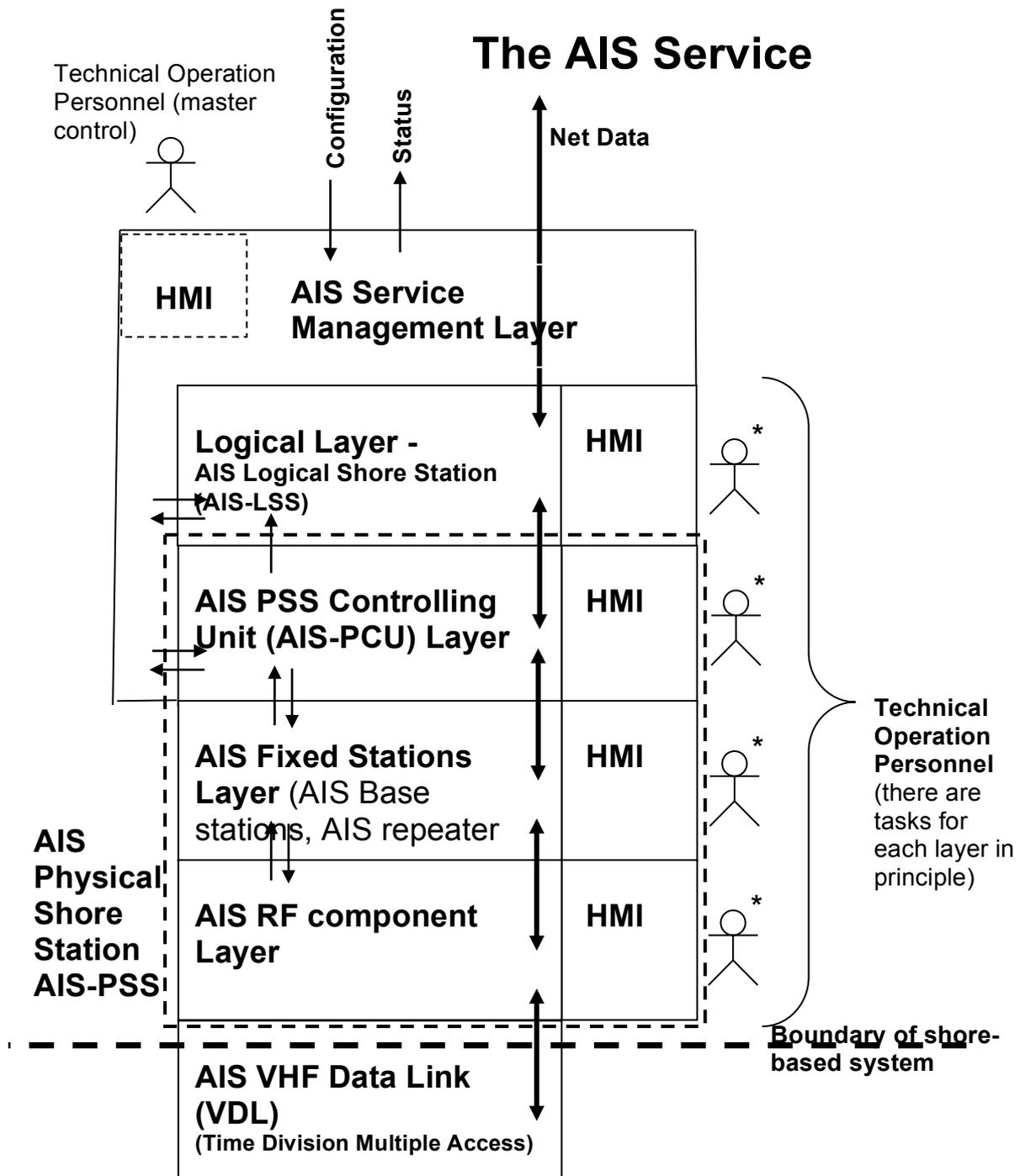
Figure 1 Layered structure of AIS Service – Structure model of the AIS Service
