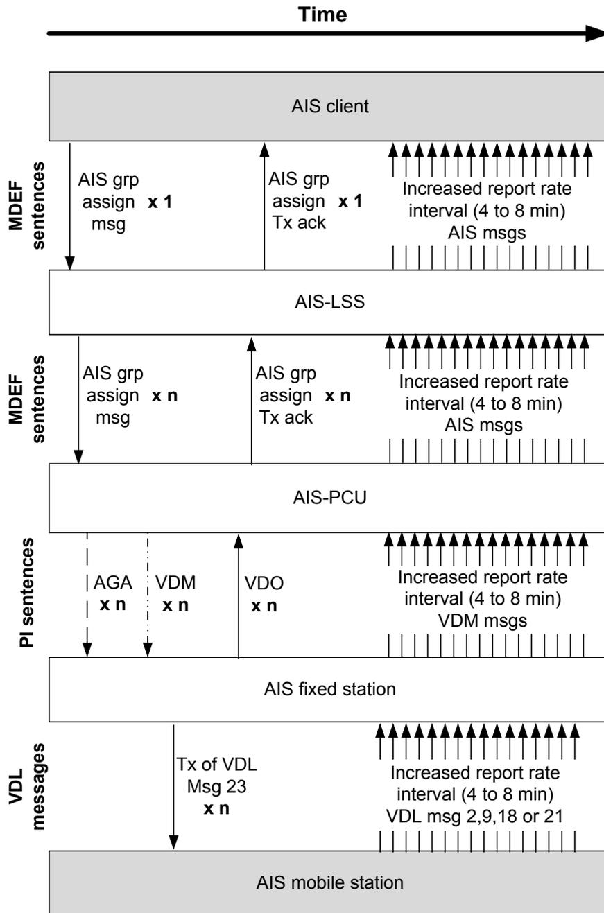
Figure 19 Interaction & data flow model for external BAS ASGN\_GROUP
