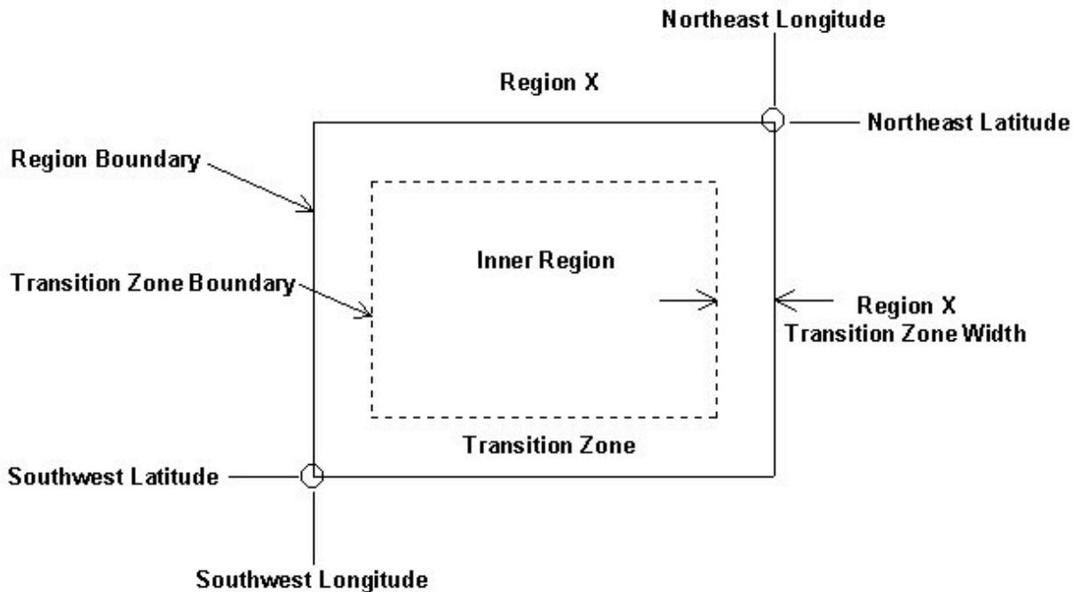
Figure 1 Rectangular representation of a region and its components
