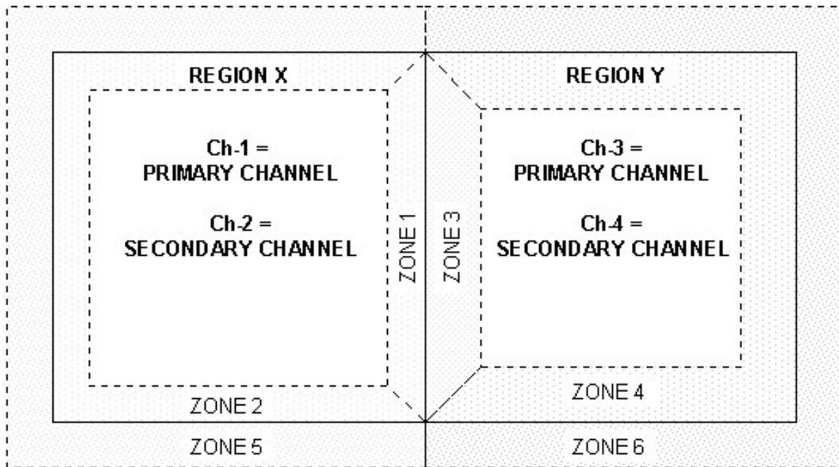
*Figure 3 Breakdown of operating zones for two adjacent regions*
